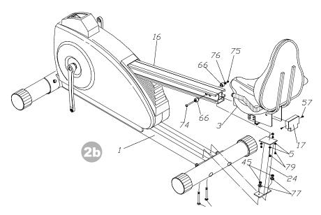
**2b.** First remove the support tube (24) from the main frame (1). Slide the assembled seat carriage onto the carriage tube (16). Re-assemble the support tube (24). Attach the end cap (17) with screws (57) and rear carriage tube rubber stopers (66) with bolts (74, 75) and washer (76).
